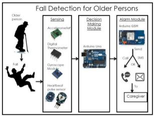
Fig.1 Components of the RAFDS
