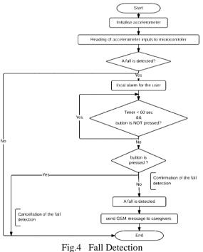
The fall detection system, shown in figure 4, starts by the accelerometer that keeps sensing the acceleration of the user and inputting the value to the microcontroller. Then, the microcontroller decides if a fall occurs based on some thresholds. The fall is detected by detecting the state of weightlessness that occurs while the body is in a free fall. This state can be detected using accelerometers, as will be discussed in the implementation section.
